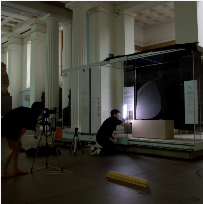
Using a novel method to capture a high-resolution normal map of the Rosetta Stone for the 3D model of the museum.
